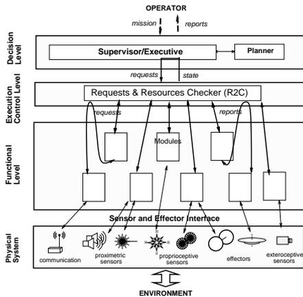
Figure 1: The LAAS Architecture.
