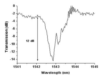
Figure 4 Transmission spectrum for the half-apodized filter
