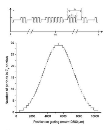
**Figure 1** Sampled grating design: schematic view (top) and Gaussian distribution of  $Z_1$  sections
