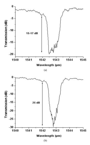
**Figure 5** Measured transmission spectra of apodized Bragg grating filter (half), with light injection from the dense grating side (b) and the other side (a)
