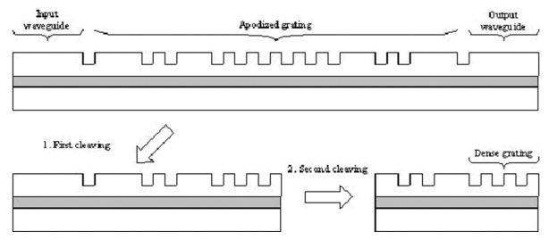
Figure 3 Schemes of the entire and cleaved apodization filters tested
