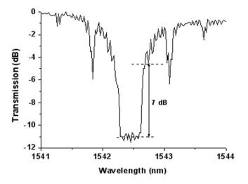
Figure 2 Measured transmission spectrum for 5-mm-long uniform filter
