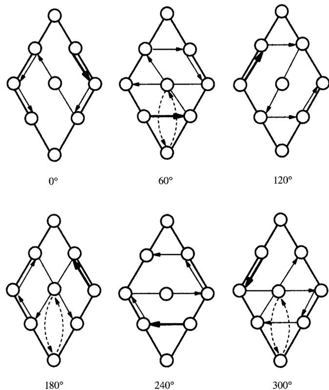
**Figure 7** Distribution of the six  $X$  rows along the edges of the minimal rhombus as a function of the rotation of the minimal rhombus itself. The arrows indicate the reading sequence corresponding to the rotation angle given below the rhombus. The two  $D$  rows are unchanged for  $\pm 120^\circ$  but exchanged for  $\pm 60$  or  $180^\circ$  rotations.
