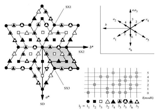
Figure 11 Construction of the star polygon corresponding to the diffraction patterns in Figs. 7–10 (see Fig. 6). The shaded minimal rhombus corresponds to the  $Z_T = \frac{3}{4}$  minimal rhombus tabulated in Nespolo *et al.* (2000).
