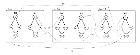
Figure 4: Periodic Register Allocation with One Reuse Circuit
