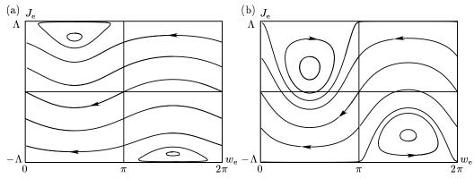
FIGURE 7. Orbits of the averaged Hamiltonian (100) restricted to the plane perpendicular to **B**. (a) shows a case with B < F, and (b) shows a case with F < B. There are two types of orbits, those which cross the lines  $w_e = 0$  and  $\pi$ , and those which oscillate around  $w_e = \frac{\pi}{2}$  and  $\frac{3\pi}{2}$ . The second type will not appear on a Poincaré section at  $w_e = 0$ .
