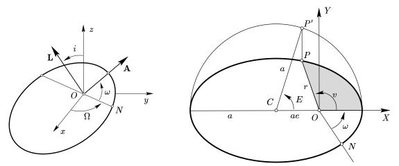
FIGURE 1. Definition of Delaunay variables. The angles  $\Omega$ , i and  $\omega$  determine the position of the Kepler ellipse in space. The line of nodes ON is the intersection of the plane of the ellipse with the xy-plane. The shaded area is proportional to the mean anomaly M. The true anomaly v and eccentric anomaly E are auxiliary quantities, allowing to relate the (X, Y)-coordinates of the planet P with M.
