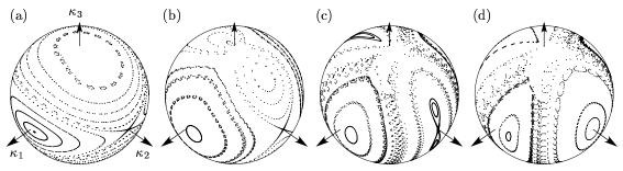
FIGURE 12. Poincaré sections at  $w_e = \frac{\pi}{2}$  of the averaged system, represented on the sphere  $\kappa_1^2 + \kappa_2^2 + \kappa_3^2 = (\Lambda - |J_e|)^2$  for increasing values of  $\frac{B}{F}$ , compare Fig. 6. In all cases,  $\Lambda = 1$ ,  $\langle H \rangle_{\Lambda} = -\frac{1}{2} - \frac{3}{2}F$ , and B = 0.1. (a) F = 0.1, (b) F = 0.05, (c) F = 0.038 and (d) F = 0.03. Points are sparse near the poles, as we only plot points obtained with sufficient numerical accuracy.
