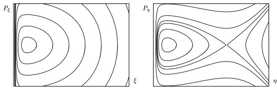
FIGURE 5. Level lines of the constants of motion  $\alpha_1$  and  $\alpha_2$  for H = 1,  $K = \frac{1}{2}$  and F = 0.05. In contrast to  $\xi$ ,  $\eta$  may have an unbounded motion. However, the saddle point is located quite far away from the origin, at  $\eta^2 = \mathcal{O}(F^{-1})$ .
