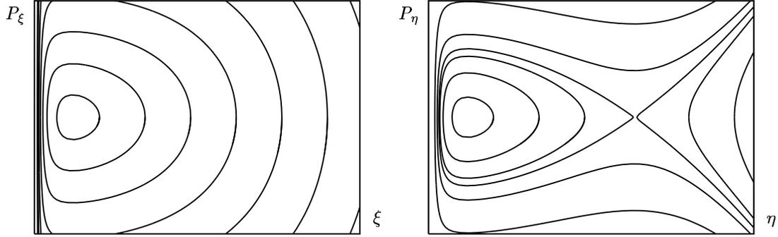
FIGURE 5. Level lines of the constants of motion  $\alpha_1$  and  $\alpha_2$  for  $H = 1$ ,  $K = \frac{1}{2}$  and  $F = 0.05$ . In contrast to  $\xi$ ,  $\eta$  may have an unbounded motion. However, the saddle point is located quite far away from the origin, at  $\eta^2 = \mathcal{O}(F^{-1})$ .
