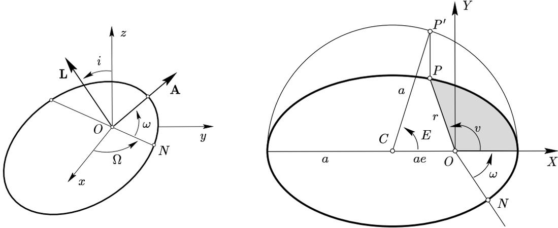
FIGURE 1. Definition of Delaunay variables. The angles  $\Omega$ ,  $i$  and  $\omega$  determine the position of the Kepler ellipse in space. The line of nodes  $ON$  is the intersection of the plane of the ellipse with the  $xy$ -plane. The shaded area is proportional to the mean anomaly  $M$ . The true anomaly  $v$  and eccentric anomaly  $E$  are auxiliary quantities, allowing to relate the  $(X, Y)$ -coordinates of the planet  $P$  with  $M$ .
