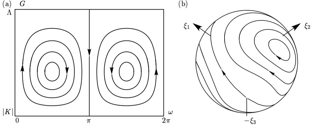
FIGURE 3. Phase portraits of the averaged Hamiltonian (36) (a) in the  $(\omega, G)$ -plane and (b) on the sphere  $\xi_1^2 + \xi_2^2 + \xi_3^2 = (\frac{1}{2}(\Lambda^2 - K^2))^2$ , seen from below the south pole. The elliptic points at  $\omega = \frac{\pi}{2}, \frac{3\pi}{2}$  correspond to periodic S-orbits of the Stark Hamiltonian.
