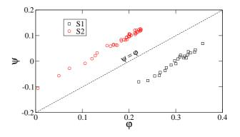
FIG. 5: Stress-dilatancy relation between dilatancy angle  $\psi$  and internal angle of friction  $\varphi$  for the samples S1 and S2.
