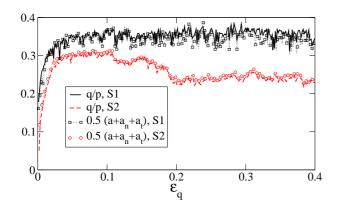
FIG. 12: Evolution of the normalized shear stress q/p for the samples S1 and S2 with  $\varepsilon_q$  together with the corresponding predictions from its expression as a function of fabric and force anisotropies [Eq. (18)].
