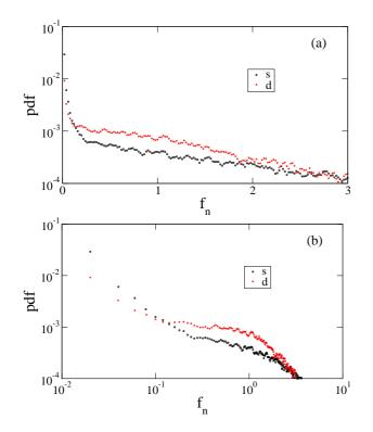
FIG. 23: Probability density function of normal forces for simple (s) and double (d) contacts in log-linear (a) and log-log scales (b).
