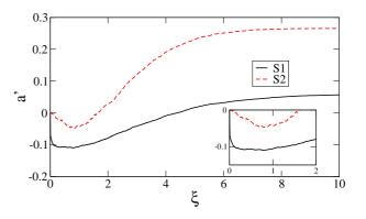
FIG. 16: Partial fabric anisotropy  $a'(\xi)$  as a function of force cutoff  $\xi$  (normalized by the mean force) in the samples S1 and S2.
