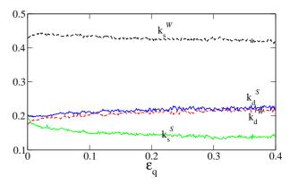
FIG. 25: Proportions  $k_s^S$  and  $k_s^W$  of strong (S) and weak (W) simple (s) contacts, respectively, as well as the proportions  $k_d^S$  and  $k_d^W$  of strong and weak double (d) contacts as a function of cumulative shear strain  $\varepsilon_q$  in the pentagon packing.
