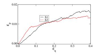
FIG. 4: Cumulative volumetric strain  $\varepsilon_p$  as a function of cumulative shear strain  $\varepsilon_q$  for the samples S1 and S2.
