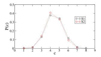
FIG. 7: Connectivity diagram for the samples S1 and S2 expressing the fraction P(c) of particles with exactly c contacts in the residual state.
