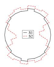
FIG. 8: Polar representation of the probability density function  $P_{\theta}$  of the contact normal directions  $\theta$  for the samples S1 and S2 in the residual state.
