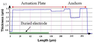
**Figure 7.** (*a*) SEM image of a parallel-plate actuator. (*b*) Close view of the nitride step covering. (*c*) Profile topography corresponding to dashed line in figure 4(a).
