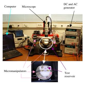
**Figure 9.** Experimental set-up. A probe station is used to keep the contact and see the motion of the actuator. A test box enables the introduction and the removal of liquid, the electrical contact is taken out of the box.
