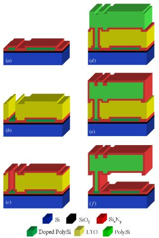
**Figure 6.** Process flow: (*a*) buried electrodes patterning; (*b*) deposition and etch of the sacrificial layer; (*c*) first level of nitride encapsulation; (*d*) deposition of the structural layer; (*e*) second level of nitride encapsulation; (*f*) releasing in a HF solution.
