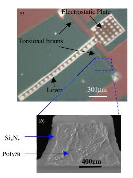
**Figure 8.** (*a*) Optical microscope image of a torsional actuator. (*b*) SEM image of cross section of the parallel-plate actuator encapsulated with  $Si_x N_y$  corresponding to the tire line in figure 5(*a*).
