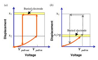
Figure 4. Displacement versus voltage characteristic for electrostatic actuation with pull-in effect (a) and without pull-in effect (b).
