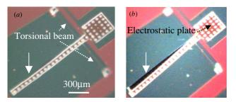
**Figure 11.** (*a*) Optical image of a torsional actuator during actuation in water when the gap is open. (*b*) Optical image of a torsional actuator during actuation when the 2  $\mu$ m gap is closed. White arrows show actuation location.
