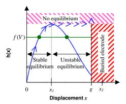
**Figure 2.** Graphic representation of equation (6). The stable equilibrium position extends from x = 0 to  $x = \min(g, x_1)$  according to (12). Arrows show the displacement of the actuator when a voltage is applied.
