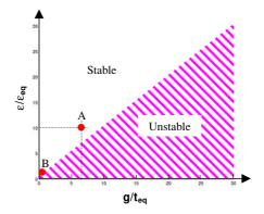
**Figure 3.** Graphical representation of condition (14). The relative permittivity is plotted versus the normalized thickness.  $t_{eq}$  and  $\varepsilon_{eq}$  are, respectively, the thickness and the permittivity of the insulating layers.
