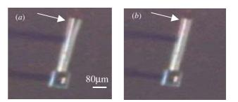
**Figure 10.** (*a*) Optical image during actuation in water when the gap is open. (*b*) Optical image during actuation in water when the 2  $\mu$ m gap is closed. White arrows show actuation location.
