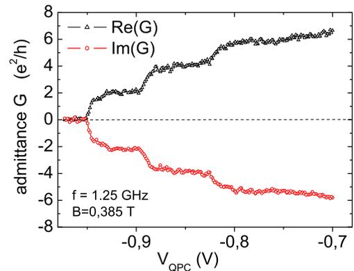
FIG. 2: Real and imaginary parts of the RF admittance of the quantum Hall conductor as function of the QPC voltage at  $T = 50mK$ . Both signals show steps at the opening of the first conducting channel. The negative imaginary part corresponds to a negative emittance which is characteristic of an inductive behavior.
