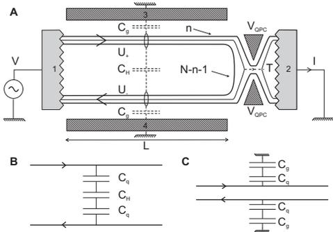
FIG. 4: A: Schematics of a quantum Hall bar with  $N$  edge states in series with a quantum point contact (QPC) with  $n$  fully transmitted channels and one partially transmitted channel. Electrochemical equivalent circuit of a Hall bar in the limit of weak edge to gate coupling (panel B) and weak interedge coupling (panel C). Notations are specified in the text.
