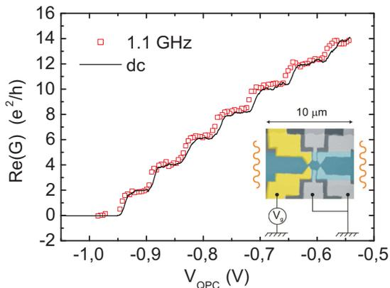
FIG. 1: Quantized steps in the dc conductance and RF transmission of the circuit as function of the QPC gate voltage. The solid line has been shifted by  $+10mV$  along the voltage axis to avoid curve overlapping which otherwise obscures figure clarity. Temperature and magnetic field are respectively  $50mK$  and  $0.224T$ .
