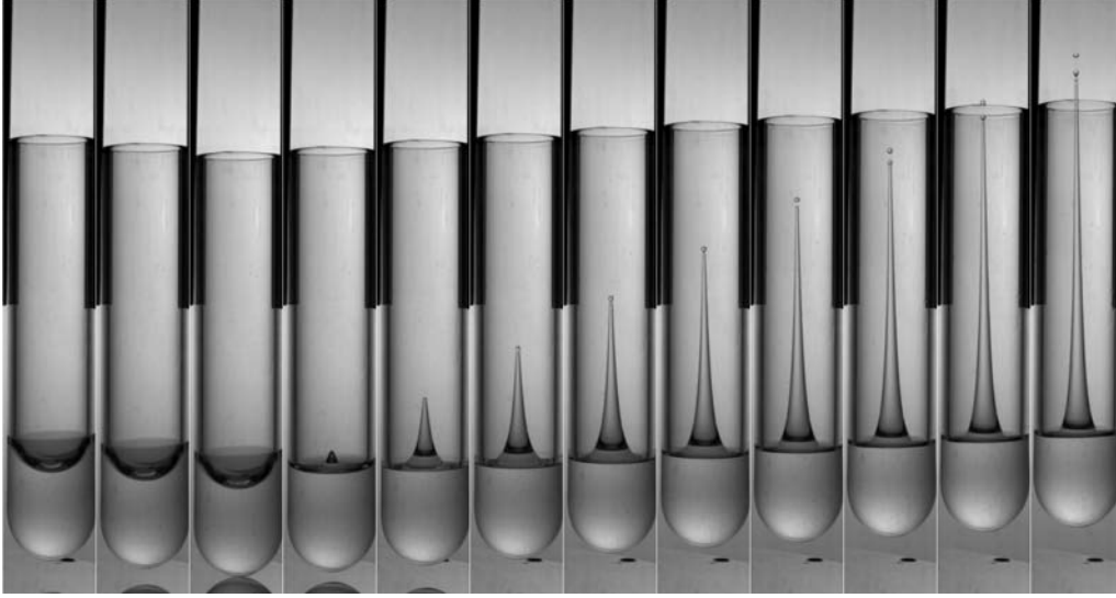
FIGURE 1. A tube filled with a wetting liquid and falling under gravity gives birth to a strong jet after impact. The interval separating each snapshot of this sequence is 5.5 ms.
