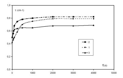
**Figure 1.** Influence of stirring rate on hydrophilic 0.5  $\mu$ m silica aggregation. 1: 200 rpm; 2: 400 rpm; 3: 800 rpm
