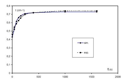
Figure 5. Comparison between experimental and simulated ( $D_f = 2.4$ ; L = 68) turbidity plots for 0.5  $\mu$ m hydrophilic silica particles aggregation at stirring rate 200 rpm.
