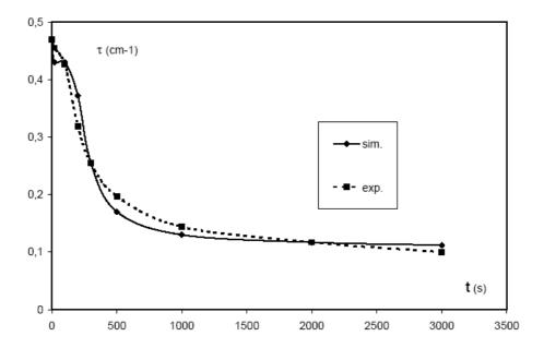
**Figure 6.** Aggregation of 0.5  $\mu$ m hydrophobic silica at 200 rpm: experimental and simulated  $(D_f = 2.67; L = 2048; P = 0.3)$  turbidity curves.
