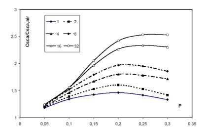
**Figure 4.** Ratio of scattering cross sections without and with gas versus gas content P for different silica aggregates (weak fractal dimension  $D_f = 2.7$ ); primary particle number per aggregate is indicated on each plot
