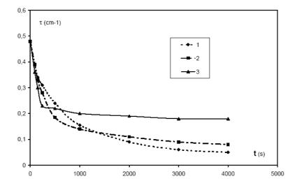
**Figure 2.** Influence of stirring rate on hydrophobic 0.5μm silica aggregation. 1: 200 rpm; 2: 400 rpm; 3: 800 rpm
