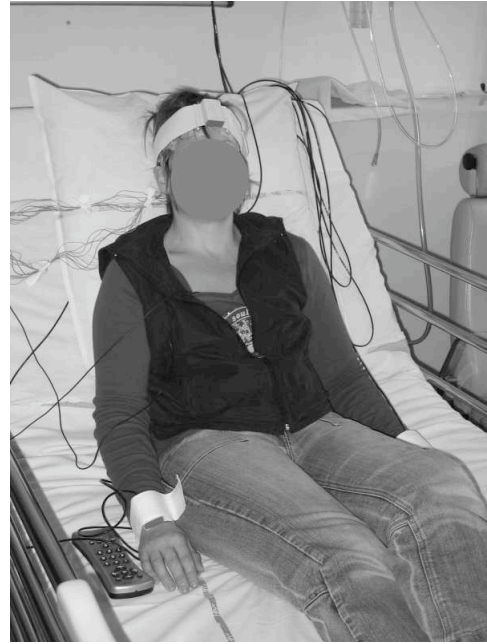
Fig. 1. Attitude sensors set on an epileptic patient. A specific design for the positioning of the sensor has been realized into flexible fabric with self gripping fasteners to be easily adjustable to the anatomy of the limb and well supported by the patient.
