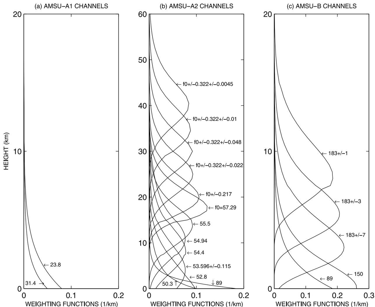
**Figure 1.** AMSU-A and AMSU-B weighting functions for a U.S. standard tropical atmosphere ( $WV = 42 \text{ kg/m}^2$ ) at nadir, assuming a surface temperature of 299 K and a surface emissivity of 0.95 for (a) AMSU-A1, (b) AMSU-A2, and (c) AMSU-B channels.
