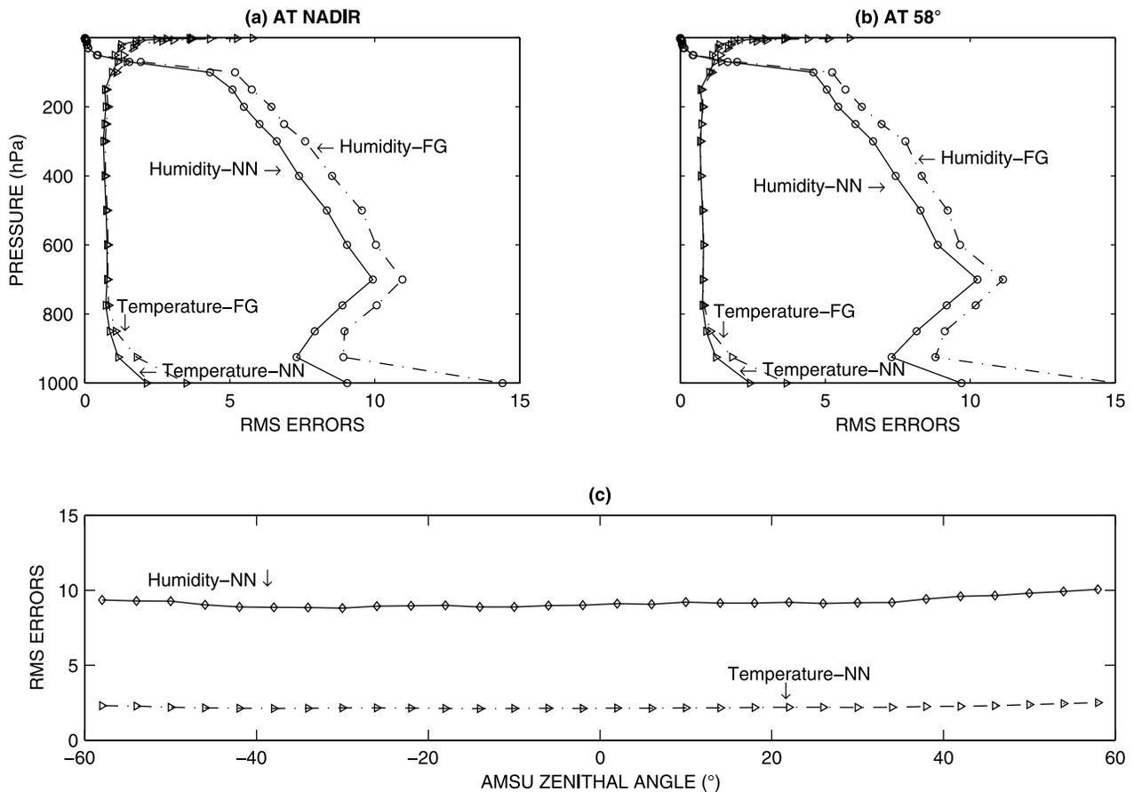
**Figure 7.** (a) Temperature and humidity RMS error profiles for nadir situations. Both FG and NN error profiles are shown. (b) Same as Figure 7a but at 58° zenith angle. (c) NN RMS errors at 1000 hPa level for both temperature and humidity sorted by AMSU zenith angle.
