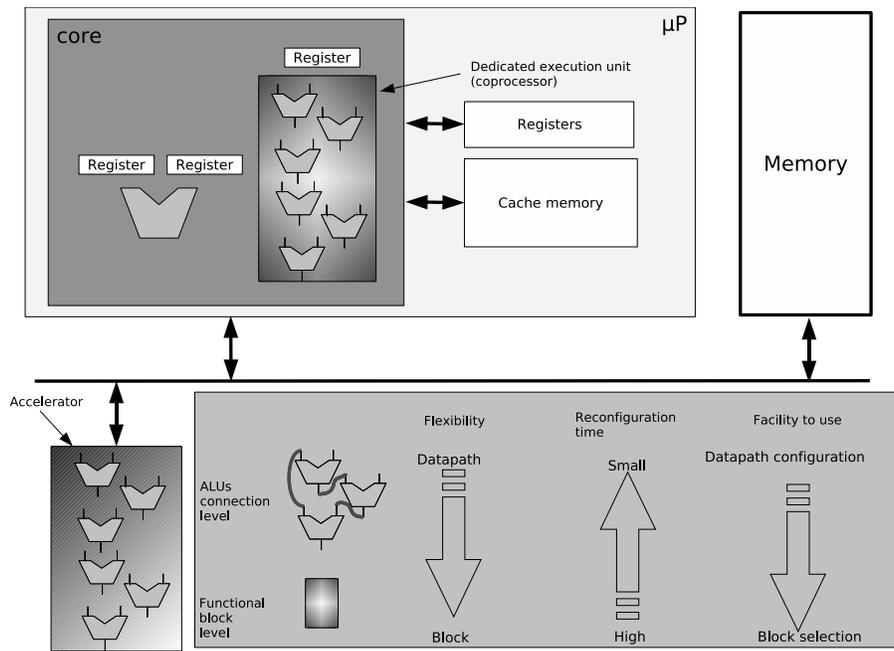
Fig. 5. Architecture with a coprocessor and an accelerator
