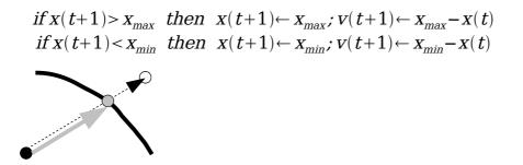
For the following confinements (4, 5, and 6) the velocity is modified so that when applied to the position we are sure that the new position is inside the search space.
