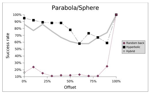
Illustration 1: Parabola/Sphere - Success rate versus (diagonal) offset
