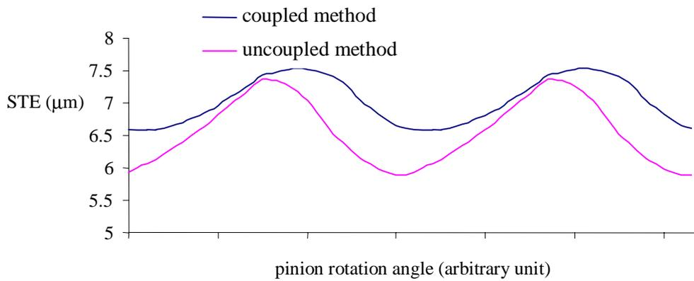
Figure 1: Static transmission error under load
