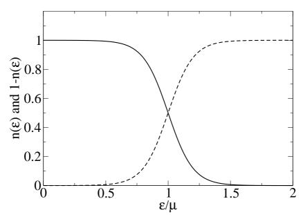
Fig. 1. – Fermi-Dirac distribution in the degenerate regime. Solid line: occupation numbers  $n(\epsilon)$ for the particles. Dashed line: occupation numbers  $1 - n(\epsilon)$  for the holes. The temperature is  $k_B T = \mu / 10.$
