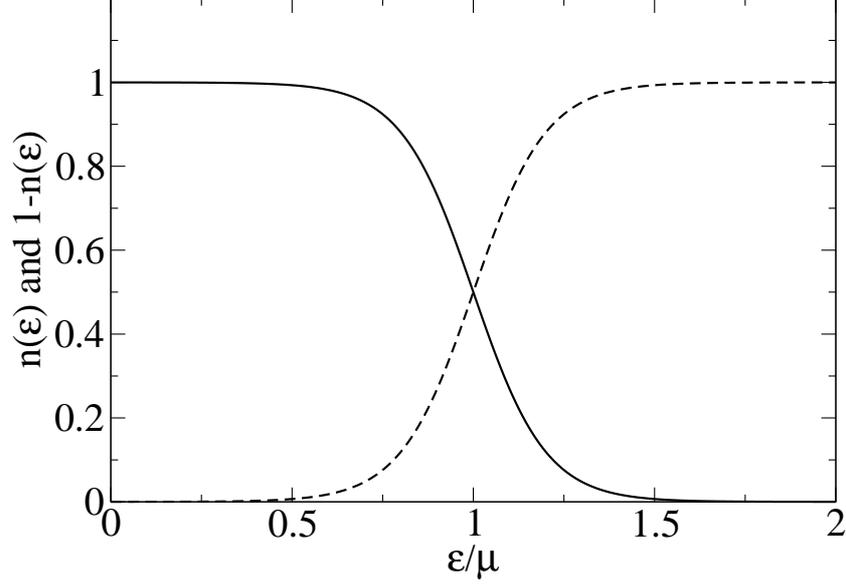
Fig. 1. – Fermi-Dirac distribution in the degenerate regime. Solid line: occupation numbers  $n(\epsilon)$  for the particles. Dashed line: occupation numbers  $1 - n(\epsilon)$  for the holes. The temperature is  $k_B T = \mu/10$ .
