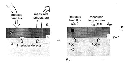
Fig. 1. – Thermography on a laminate with interfacial defects.
