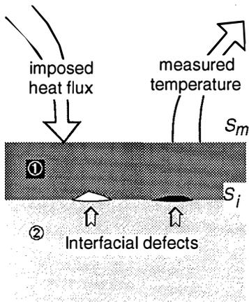
Fig. 1. - Thermography on a laminate with interfacial defects.
