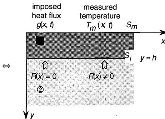
Fig. 2. - Modelisation of the interfacial defects.
