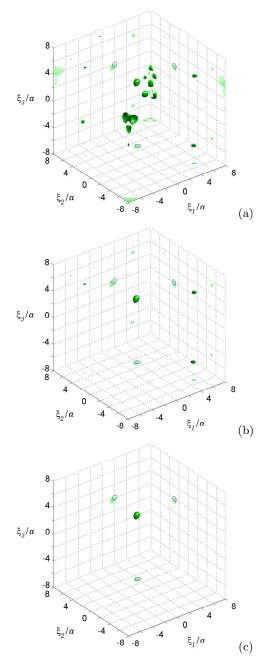
Fig. 6. Identification of spherical hard scatterer of radius 0.4a: iso-surfaces of  $\mathcal{T}(\boldsymbol{x}_s)$  for  $\mathcal{T} = 0.55\mathcal{T}_{\min}$ , computed on the entire search grid  $\mathcal{S}$  (a) and on truncated search grids such that  $\{|\xi_i| \leq 6.5a \ (i=1,2,3)\}$  (b) and  $\{|\xi_i| \leq 5a \ (i=1,2,3)\}$  (c). Values of  $\mathcal{T}(\boldsymbol{x}_s)$  lower than the iso-value are inside the iso-surface.
