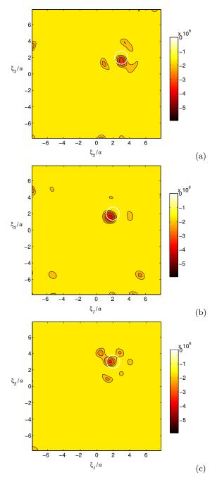
**Fig. 5.** Identification of spherical hard scatterer of radius 0.8a: distribution of thresholded topological sensitivity  $\hat{\mathcal{T}}(\boldsymbol{x}_{\mathrm{s}})$  for sampling points  $\boldsymbol{x}_{\mathrm{s}}$  in coordinate planes  $\xi_1 = x_1^{\mathrm{true}}$  (a),  $x_2 = x_2^{\mathrm{true}}$  (b) and  $x_3 = x_3^{\mathrm{true}}$  (c).
