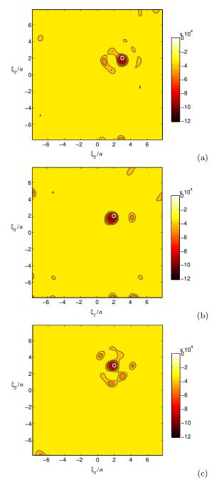
**Fig. 3.** Identification of spherical hard scatterer of radius 0.2a: distribution of thresholded topological sensitivity  $\hat{\mathcal{T}}(\boldsymbol{x}_{\mathrm{s}})$  for sampling points  $\boldsymbol{x}_{\mathrm{s}}$  in coordinate planes  $\xi_1 = x_1^{\mathrm{true}}$  (a),  $x_2 = x_2^{\mathrm{true}}$  (b) and  $x_3 = x_3^{\mathrm{true}}$  (c).
