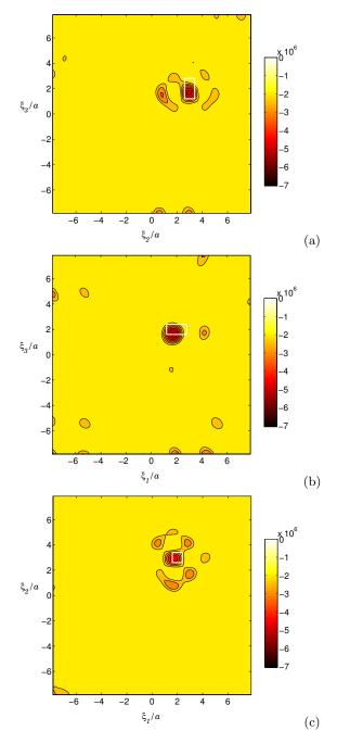
Fig. 8. Identification of box-shaped scatterer: distribution of thresholded topological sensitivity  $\hat{T}(\boldsymbol{x}_{\mathrm{s}})$  for sampling points  $\boldsymbol{x}_{\mathrm{s}}$  in coordinate planes  $\xi_{1} = x_{1}^{\mathrm{true}}$  (a),  $x_{2} = x_{2}^{\mathrm{true}}$  (b) and  $x_{3} = x_{3}^{\mathrm{true}}$  (c).
