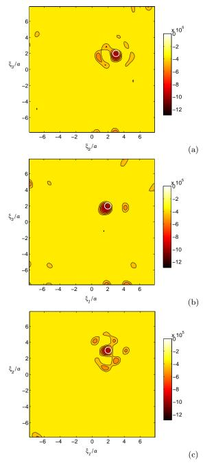
**Fig. 4.** Identification of spherical hard scatterer of radius 0.4a: distribution of thresholded topological sensitivity  $\hat{\mathcal{T}}(\boldsymbol{x}_{\mathrm{s}})$  for sampling points  $\boldsymbol{x}_{\mathrm{s}}$  in coordinate planes  $\xi_1 = x_1^{\mathrm{true}}$  (a),  $x_2 = x_2^{\mathrm{true}}$  (b) and  $x_3 = x_3^{\mathrm{true}}$  (c).
