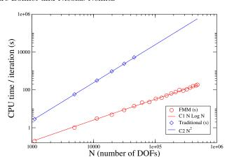
**Fig. 1.** CPU time for one evaluation of residual (40) as a function of the number N of nodal unknowns, with matrix-vector products computed using classical BEM techniques (lozenges, theoretical complexity  $O(N^2)$ ) or the FM-BEM (circles, theoretical complexity  $O(N \log N)$ ).
