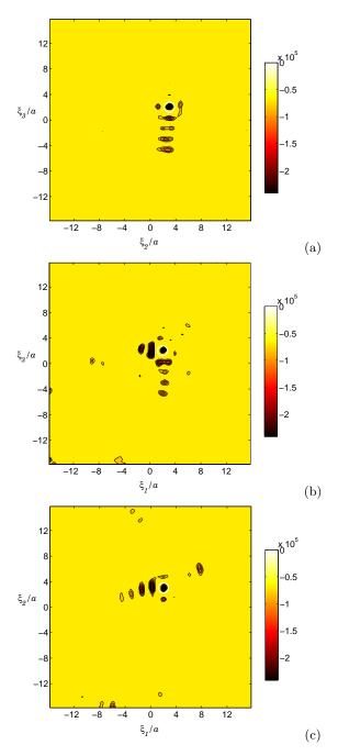
**Fig. 9.** Identification of spherical hard scatterer of radius 0.4a in large domain: distribution of thresholded topological sensitivity  $\hat{\mathcal{T}}(\boldsymbol{x}_{\mathrm{s}})$  for sampling points  $\boldsymbol{x}_{\mathrm{s}}$  in coordinate planes  $\xi_1 = x_1^{\mathrm{true}}$  (a),  $x_2 = x_2^{\mathrm{true}}$  (b) and  $x_3 = x_3^{\mathrm{true}}$  (c).
