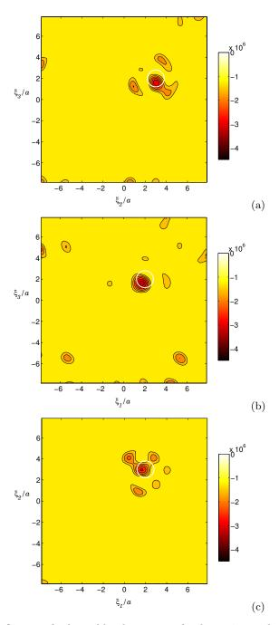
Fig. 7. Identification of spherical hard scatterer of radius 0.4a, synthetic data with 10% noise: distribution of thresholded topological sensitivity  $\hat{\mathcal{T}}(\boldsymbol{x}_{\mathrm{s}})$  for sampling points  $\boldsymbol{x}_{\mathrm{s}}$  in coordinate planes  $\xi_{1} = x_{1}^{\mathrm{true}}$  (a),  $x_{2} = x_{2}^{\mathrm{true}}$  (b) and  $x_{3} = x_{3}^{\mathrm{true}}$  (c).
