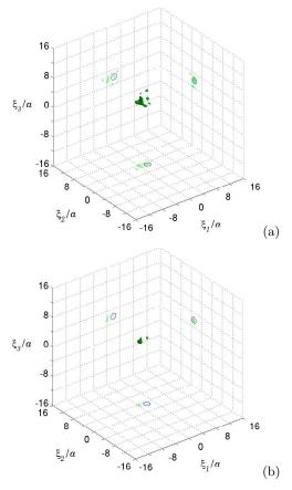
Fig. 10. Identification of spherical hard scatterer of radius 0.8a embedded in large domain  $\Omega(16a)$ : iso-surfaces of (a)  $\mathcal{T}(\boldsymbol{x}_s)$  for  $\mathcal{T}=0.55\mathcal{T}_{\min}$  and (b)  $\mathcal{T}=0.7\mathcal{T}_{\min}$  computed on the truncated search grid such that  $\{|\xi_i| \leq 14a \ (i=1,2,3)\}$ . Values of  $\mathcal{T}(\boldsymbol{x}_s)$  lower than the iso-value are inside the iso-surface.
