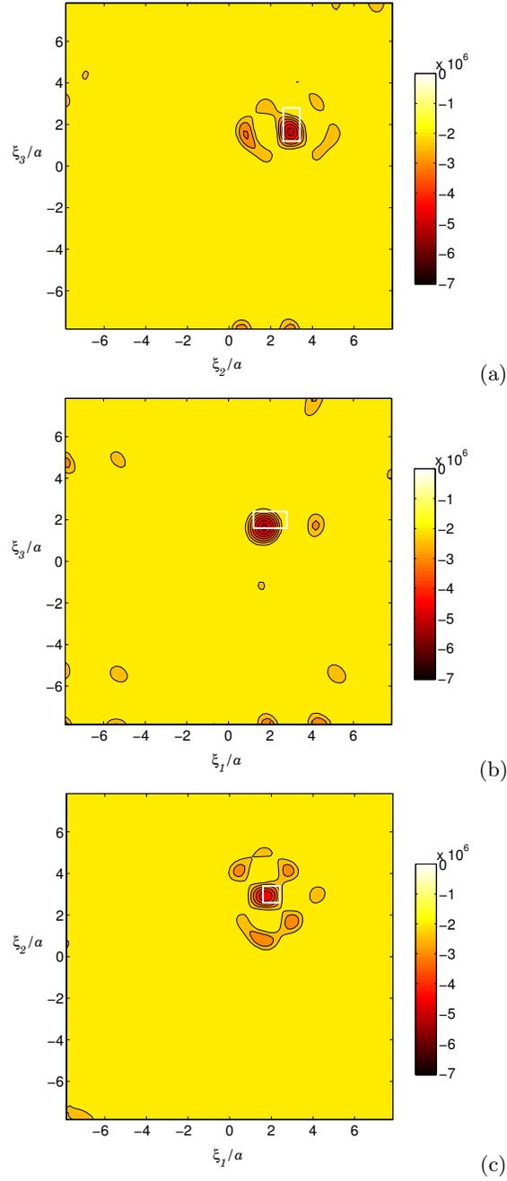
**Fig. 8.** Identification of box-shaped scatterer: distribution of thresholded topological sensitivity  $\hat{\mathcal{T}}(\mathbf{x}_s)$  for sampling points  $\mathbf{x}_s$  in coordinate planes  $\xi_1 = x_1^{\text{true}}$  (a),  $x_2 = x_2^{\text{true}}$  (b) and  $x_3 = x_3^{\text{true}}$  (c).
