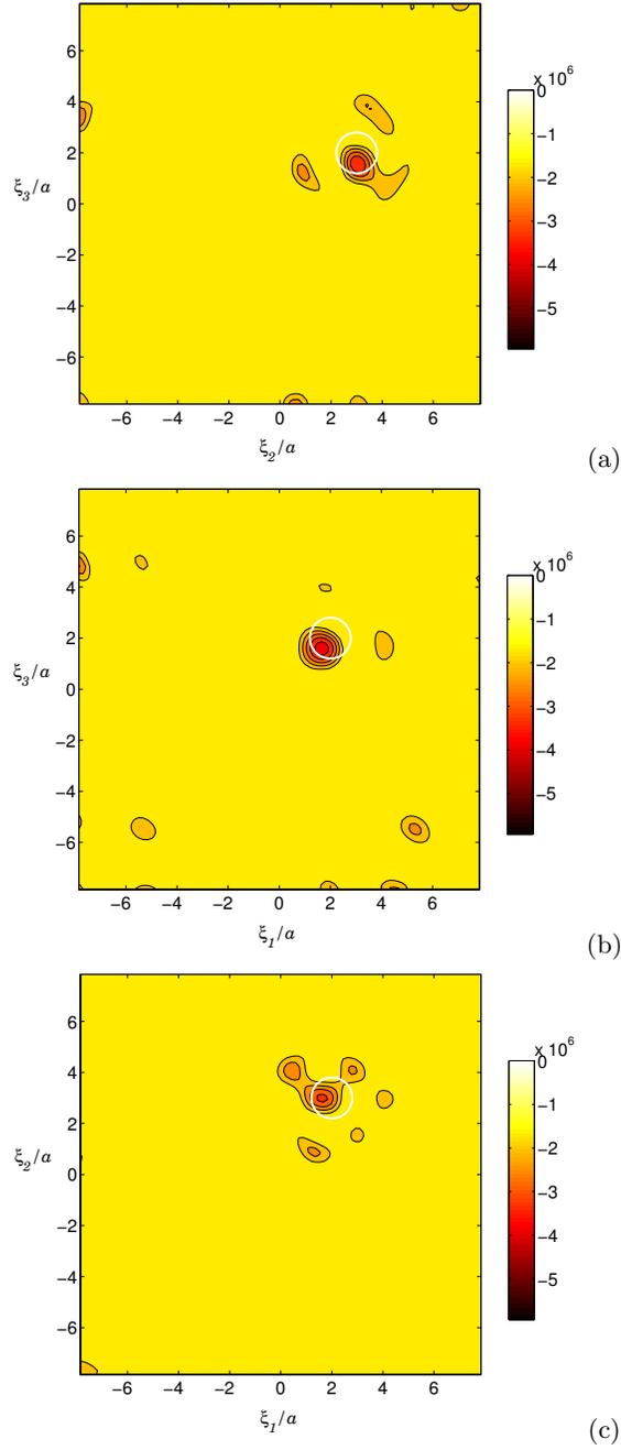
**Fig. 5.** Identification of spherical hard scatterer of radius  $0.8a$ : distribution of thresholded topological sensitivity  $\tilde{T}(\mathbf{x}_s)$  for sampling points  $\mathbf{x}_s$  in coordinate planes  $\xi_1 = x_1^{\text{true}}$  (a),  $x_2 = x_2^{\text{true}}$  (b) and  $x_3 = x_3^{\text{true}}$  (c).
