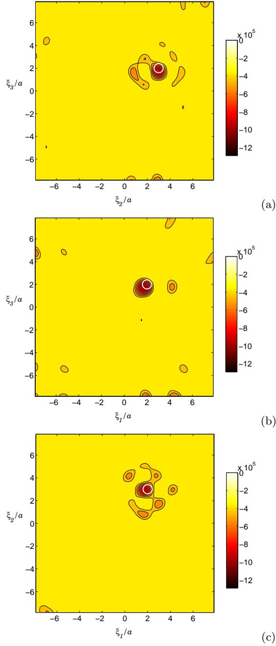
**Fig. 4.** Identification of spherical hard scatterer of radius  $0.4a$ : distribution of thresholded topological sensitivity  $\tilde{\mathcal{I}}(\mathbf{x}_s)$  for sampling points  $\mathbf{x}_s$  in coordinate planes  $\xi_1 = x_1^{\text{true}}$  (a),  $x_2 = x_2^{\text{true}}$  (b) and  $x_3 = x_3^{\text{true}}$  (c).
