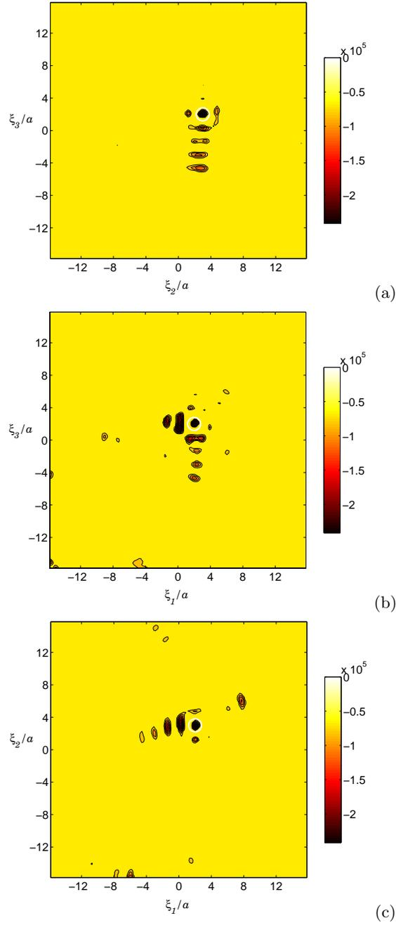
**Fig. 9.** Identification of spherical hard scatterer of radius  $0.4a$  in large domain: distribution of thresholded topological sensitivity  $\tilde{T}(\mathbf{x}_s)$  for sampling points  $\mathbf{x}_s$  in coordinate planes  $\xi_1 = x_1^{\text{true}}$  (a),  $x_2 = x_2^{\text{true}}$  (b) and  $x_3 = x_3^{\text{true}}$  (c).
