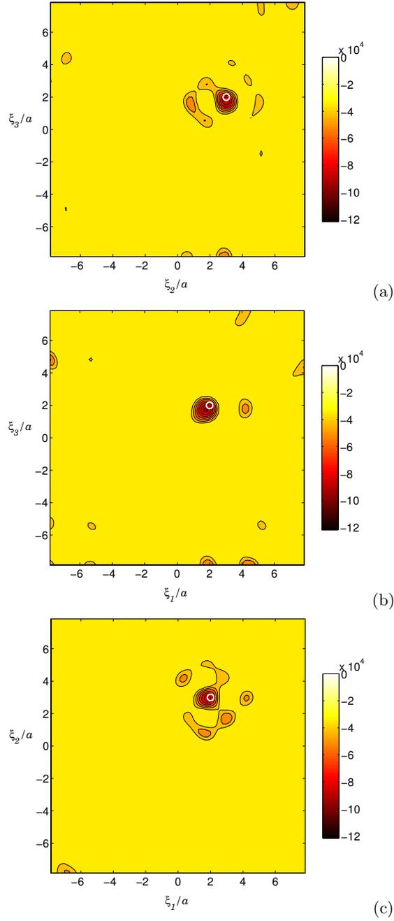
**Fig. 3.** Identification of spherical hard scatterer of radius  $0.2a$ : distribution of thresholded topological sensitivity  $\tilde{\mathcal{I}}(\mathbf{x}_s)$  for sampling points  $\mathbf{x}_s$  in coordinate planes  $\xi_1 = x_1^{\text{true}}$  (a),  $x_2 = x_2^{\text{true}}$  (b) and  $x_3 = x_3^{\text{true}}$  (c).
