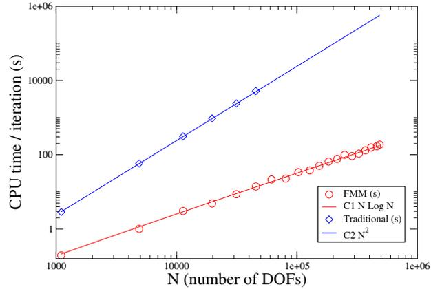
**Fig. 1.** CPU time for one evaluation of residual (40) as a function of the number  $N$  of nodal unknowns, with matrix-vector products computed using classical BEM techniques (lozenges, theoretical complexity  $O(N^2)$  or the FM-BEM (circles, theoretical complexity  $O(N\text{Log}N)$ ).
