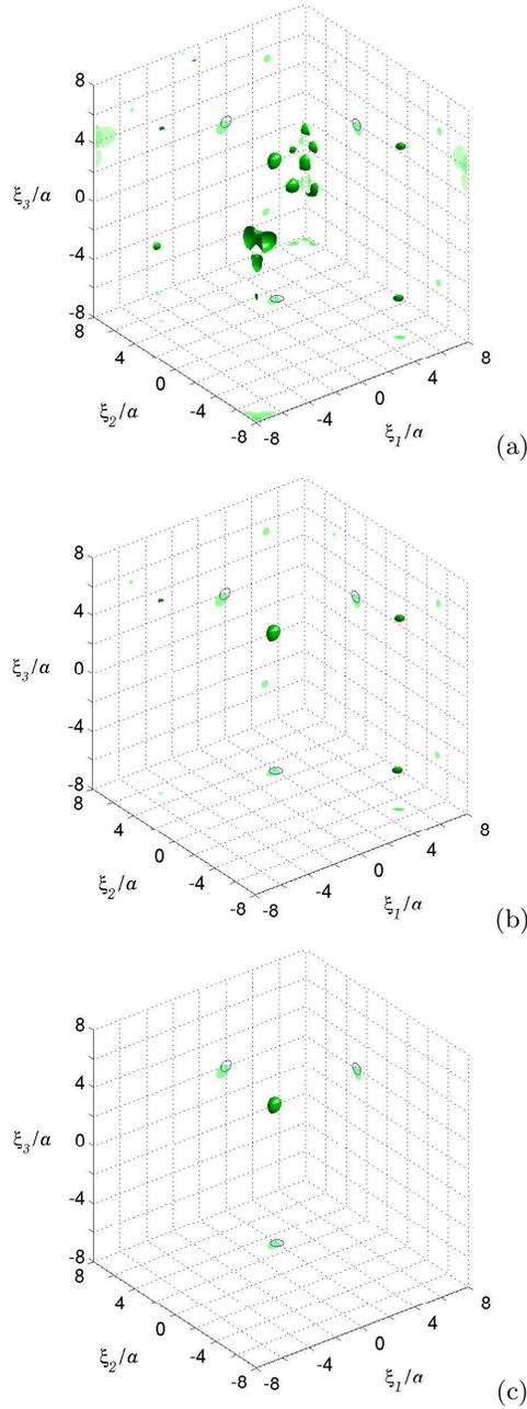
**Fig. 6.** Identification of spherical hard scatterer of radius  $0.4a$ : iso-surfaces of  $\mathcal{T}(\mathbf{x}_s)$  for  $\mathcal{T} = 0.55\mathcal{T}_{\min}$ , computed on the entire search grid  $\mathcal{S}$  (a) and on truncated search grids such that  $\{|\xi_i| \leq 6.5a \ (i=1, 2, 3)\}$  (b) and  $\{|\xi_i| \leq 5a \ (i=1, 2, 3)\}$  (c). Values of  $\mathcal{T}(\mathbf{x}_s)$  lower than the iso-value are inside the iso-surface.
