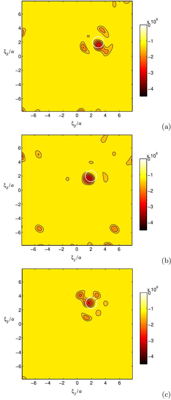
**Fig. 7.** Identification of spherical hard scatterer of radius  $0.4a$ , synthetic data with 10% noise: distribution of thresholded topological sensitivity  $\hat{T}(\mathbf{x}_s)$  for sampling points  $\mathbf{x}_s$  in coordinate planes  $\xi_1 = x_1^{\text{true}}$  (a),  $x_2 = x_2^{\text{true}}$  (b) and  $x_3 = x_3^{\text{true}}$  (c).
