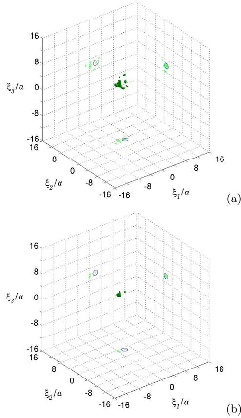
**Fig. 10.** Identification of spherical hard scatterer of radius  $0.8a$  embedded in large domain  $\Omega(16a)$ : iso-surfaces of **(a)**  $\mathcal{T}(\mathbf{x}_s)$  for  $\mathcal{T} = 0.55\mathcal{T}_{\min}$  and **(b)**  $\mathcal{T} = 0.7\mathcal{T}_{\min}$  computed on the truncated search grid such that  $\{|\xi_i| \leq 14a \ (i = 1, 2, 3)\}$ . Values of  $\mathcal{T}(\mathbf{x}_s)$  lower than the iso-value are inside the iso-surface.
