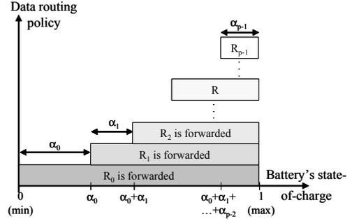
Figure 1. Priority-based packet forwarding at the intermediate nodes
