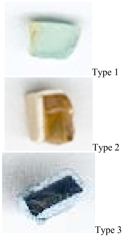
Fig. 4 : Sample sections after 20 h thermal treatment in sulfuric acid for the different type of glass.
