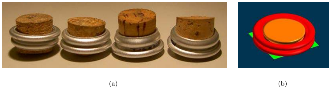
Figure 22: Samples geometry after 15 m/s impact – (a) experimental – (b) numerical.
