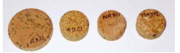
Figure 6: Cork samples tested with SHPB.
