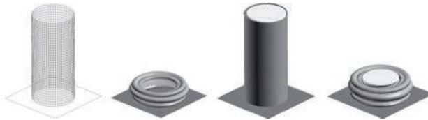
Figure 3. Shape histories of the tubes simulated (empty tubes on the left, cork-filled [CF] on the right).
