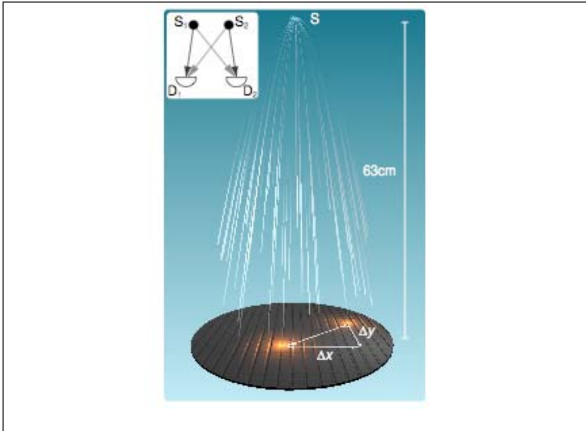
Caption for figure 1: The experimental setup. A cold cloud of metastable helium atoms is released at the switch-off of a magnetic trap. The cloud expands and falls under the effect of gravity onto a time resolved and position sensitive detector (micro-channel plate and delay-line anode), that detects single atoms. The inset shows conceptually the two 2-particle amplitudes (in black or grey) that interfere to give bunching or antibunching: S_1 and S_2 refer to the initial positions of two identical atoms jointly detected at D_1 and D_2 .
