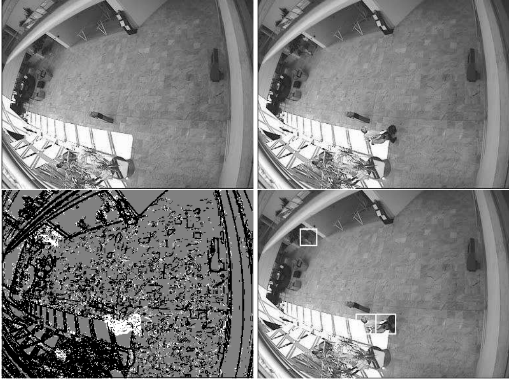
FIGURE 1: Top left, the reference background B , on its left the image I , bottom left the difference image and, bottom right, the maximal meaningful windows.
