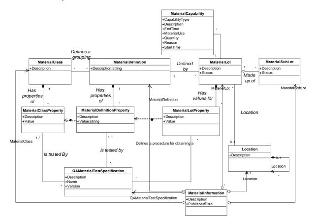
Figure 6: The conceptualised IEC 62264 Material model
