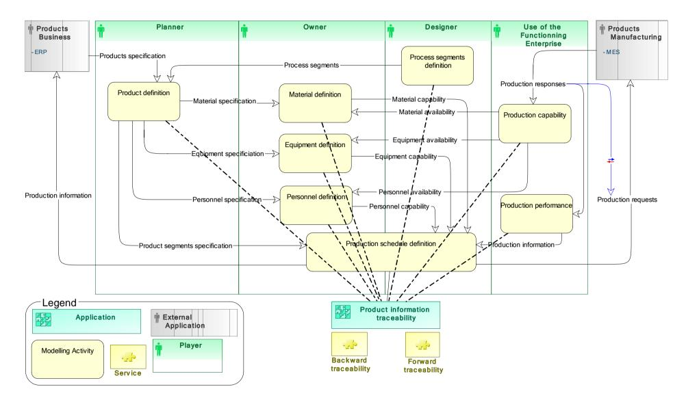
Figure 12: The IEC 62264 modelling framework workflow
