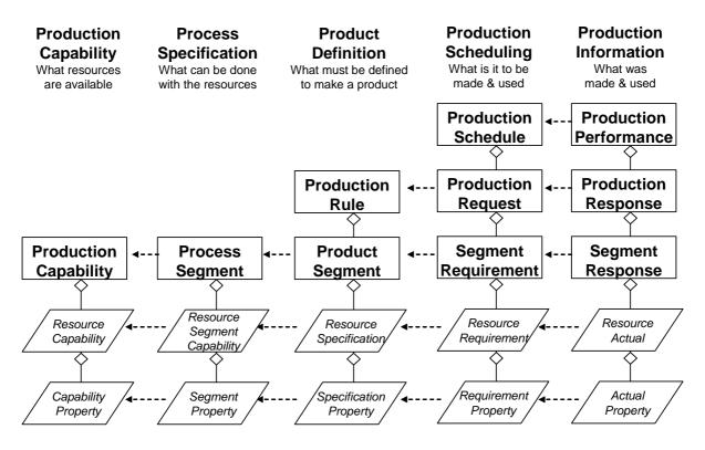
Figure 3: The IEC 62264 models hierarchy (IEC 62264, 2002)
