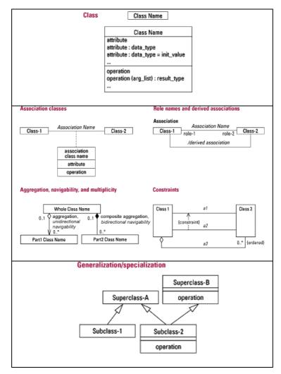
Figure 4: The UML class diagram formalism
