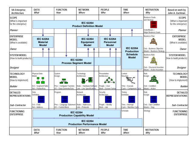
Figure 10: IEC 62264 models mapped onto the Zachman framework players view Let us now explain, line by line, model by model, what our mapping will bring. In Figure 10, the arrows have the semantics of "*has a reference to*"; for example, the "Product Definition Model" has references to the "Material Model", the "Equipment Model", the "Personnel Model" and the "Process Segment Model".
