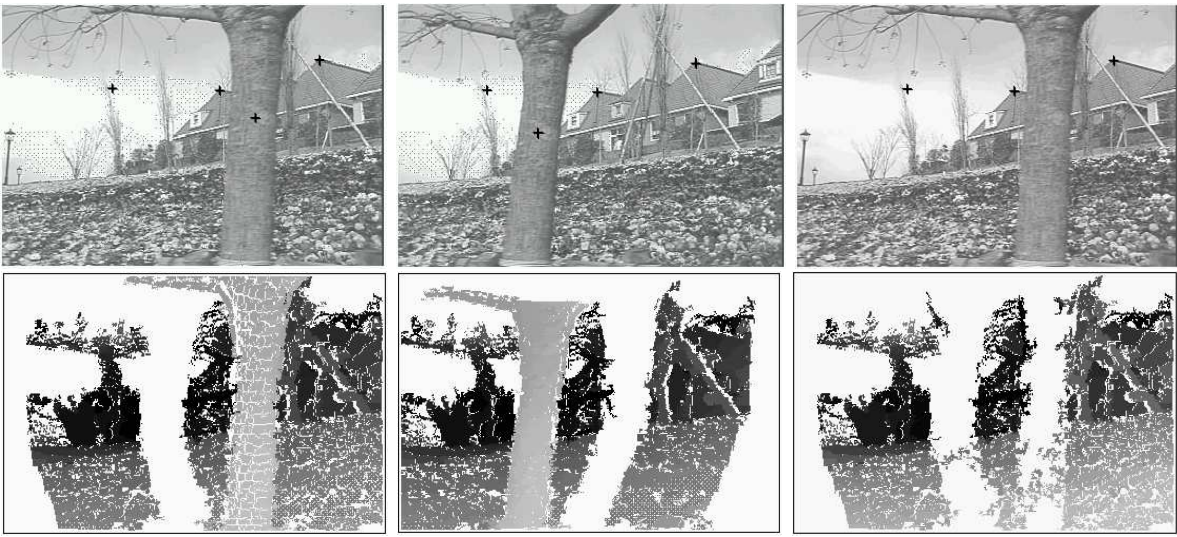
Figure 5: The disparity maps produced by propagation with different seed points and without the epipolar constraint. Left and Middle columns: four manually selected seed points marked by a cross between the 1st and the 20th frame of the flower garden. Right column: remove one manual seed located on the front tree. It has more match outliers in the occluded regions.
