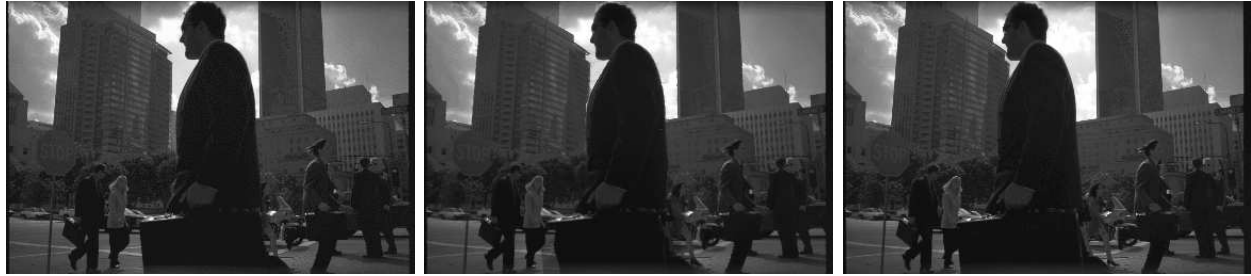
Figure 18: A typical usage of virtual vertices from the original image sequence. The fast-moving foreground man with slowly moving background buildings creates the half-occluded areas between the man and the building: The original images are on the left and right and the interpolated image is in the middle.
