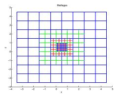
FIGURE 1. Dyadic mesh for a periodic domain in two direction  $(8 \times 8 \times 8 \text{ mesh of the core domain})$ .
