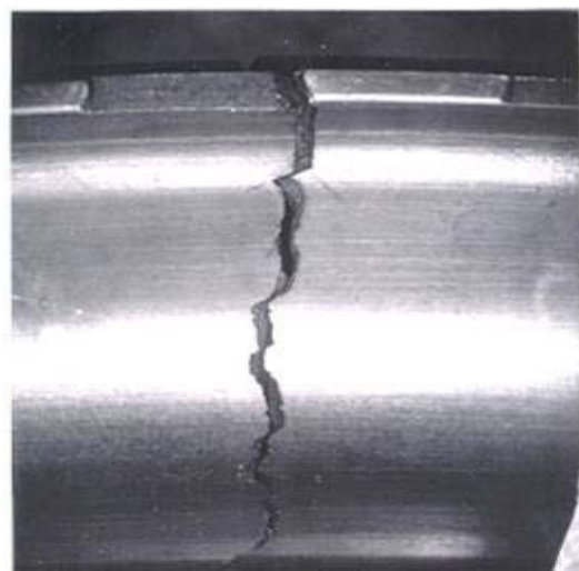
Figure 2. Fretting fatigue induced failure on a casing flange.
