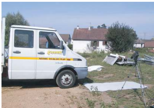
Figure 5. Heavy wheeled vehicle used as moving loading system on 3D-woven polyester mats.
