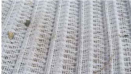
Figure 4. 3D-woven polyester mat lying on soil.
