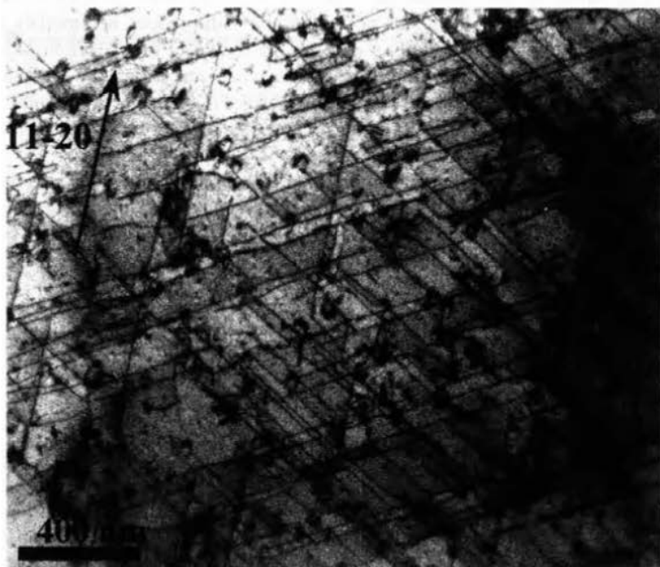
FIG. 9—Deformation mechanisms at T < 200^{\circ}\text{C} : a) prismatic slip plane traces (SEM), b) long screw \langle a \rangle type dislocations (TEM: basal projection).
