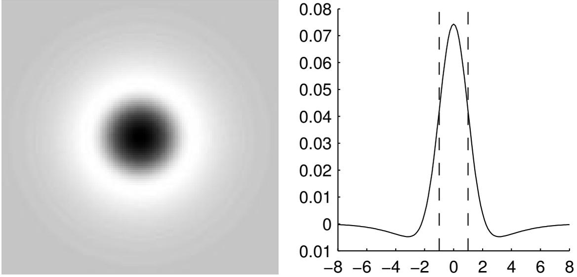
Figure 5: **Mother function for the filters in the retina.** (*Left*) The DOG filter is a center-OFF (in black) surround-ON (in white) contrast detector. (*Right*) Central profile of the DOG filter. As a unit measure, the vertical striped lines represent the variance of the narrower Gaussian used to generate the DOG filter and thus corresponds to the center of neighboring filters.
