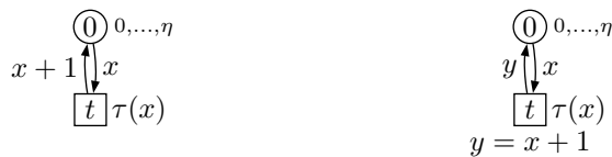
FIG. 2.1. On the left, a Petri net which actually denotes that given on the right, with \eta \geq 0 , \{0, \dots, \eta\} \subseteq \mathbb{D} , \{x, y\} \subseteq \mathbb{V} and \tau \in \mathbb{S} .
