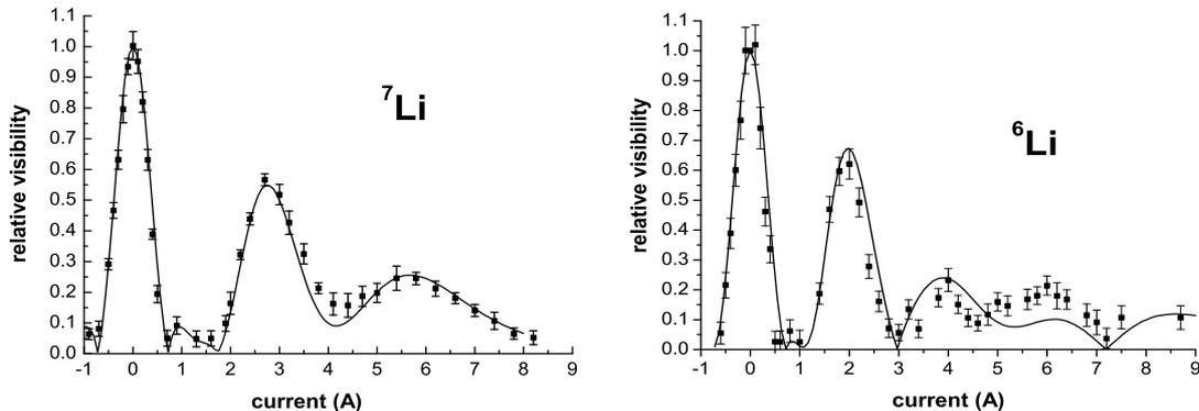
Fig. 3 – Relative visibility  $\mathcal{V}_r$  as a function of the applied current for  ${}^7\text{Li}$  (left panel) and  ${}^6\text{Li}$  (right panel). Experimental data points are represented by dots and the fits by full curves.
