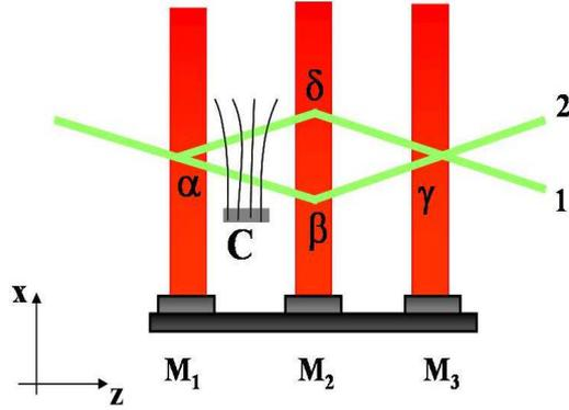
Fig. 1 – Schematic drawing of our Mach-Zehnder atom interferometer: a collimated atomic beam is diffracted by three laser standing waves, produced by reflecting three laser beams on three mirrors  $M_i$ . The output beams labelled 1 and 2 are complementary, one of them (usually beam 1) being detected. A coil  $C$  close to the atomic beams creates a magnetic field gradient in the  $\mathbf{x}$ -direction.
