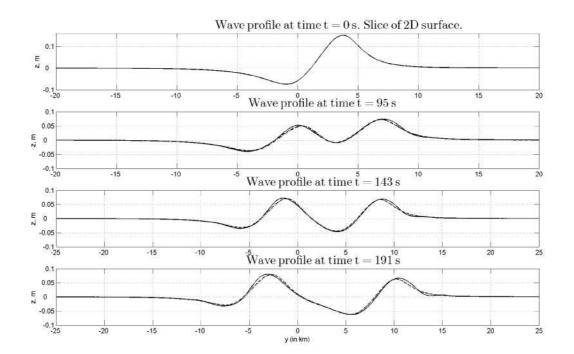
Figure 6: Comparisons of the free-surface elevation at x=0 resulting from the integration of the linear equations  $(\cdots)$ , NSW equations (--) and non-linear equations (-) at different times of the propagation of transient waves generated by an earthquake (t=0 s, t=95 s, t=143 s, t=191 s). The parameters for the earthquake are those given in Table 1. The water depth is h=100 m. One has the following estimates:  $\varepsilon=5\times10^{-4}, \ \mu^2=10^{-4}$  and consequently S=5.
