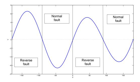
Figure 3: Initial net volume V (in km<sup>3</sup>) of the seafloor displacement as a function of the dip angle  $\delta$  (in °). All the other parameters, which are given in Table 1, are kept constant.
