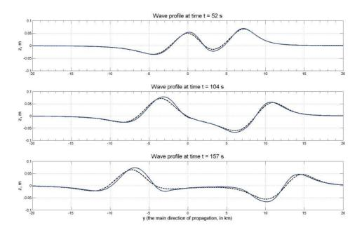
Figure 7: Comparisons of the free-surface elevation at x=0 resulting from the integration of the linear equations  $(\cdots)$ , NSW equations (--) and non-linear equations (-) at different times of the propagation of transient waves generated by an earthquake (t=52 s, t=104 s, t=157 s). The parameters for the earthquake are those given in Table 1. The water depth is h=500 m. One has the following estimates:  $\varepsilon=10^{-4}$ ,  $\mu^2=2.5\times10^{-3}$  and consequently S=0.04.
