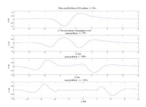
Figure 4: Wave profiles at different times for the case of a normal fault  $(\delta = 167^{\circ})$ . The seafloor deformation occurs instantaneously at t = 0. The water depth h(x, y) is assumed to be constant.
