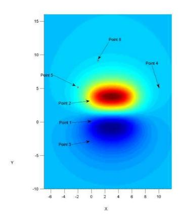
Figure 8: Top view of the initial free surface deformation showing the location of six selected gauges, with the following coordinates (in km): (1) 0.0; (2) 0.3; (3) 0.-3; (4) 10.5; (5) -2.5; (6) 1.10. The lower oval area represents the initial subsidence while the upper oval area represents the initial uplift.
