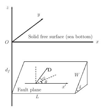
Figure 1: Geometry of the source model (dip angle  $\delta$ , depth  $d_f$ , length L, width W) and orientation of Burger's vector  $\mathbf{D}$  (rake angle  $\theta$ , angle  $\phi$  between the fault plane and Burger's vector).
