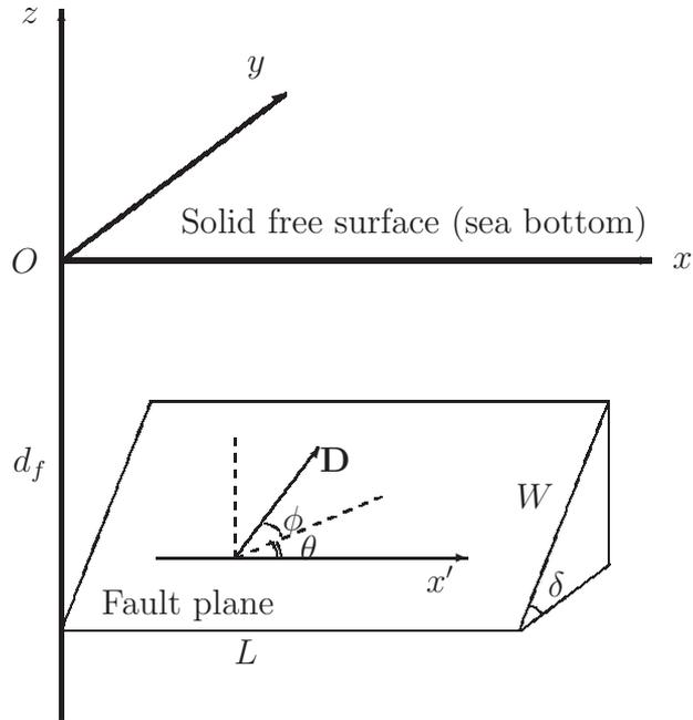
Figure 1: Geometry of the source model (dip angle  $\delta$ , depth  $d_f$ , length  $L$ , width  $W$ ) and orientation of Burger's vector  $\mathbf{D}$  (rake angle  $\theta$ , angle  $\phi$  between the fault plane and Burger's vector).
