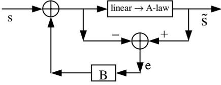
Figure 4: Noise shaping using a feedback loop.
