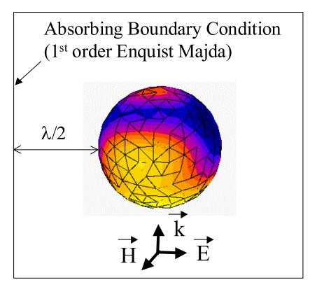
Figure 1 : H field modulus on a PEC sphere
