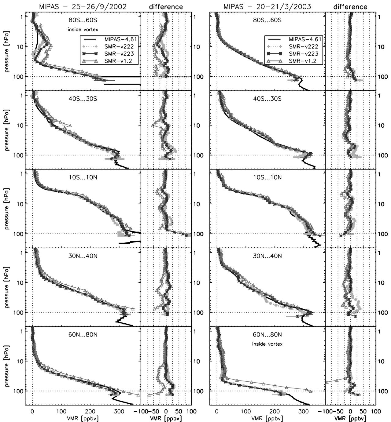
**Figure 13.** (left) Comparison of zonal mean N<sub>2</sub>O from Odin/SMR for 25–26 September 2002 (1200–1200 UT) for selected latitude bands with zonal means derived from measurements of the MIPAS instrument on board the Envisat satellite for the same period (v4.61 off-line data). (right) Same but for 20–21 March 2003 (1200–1200 UT).
