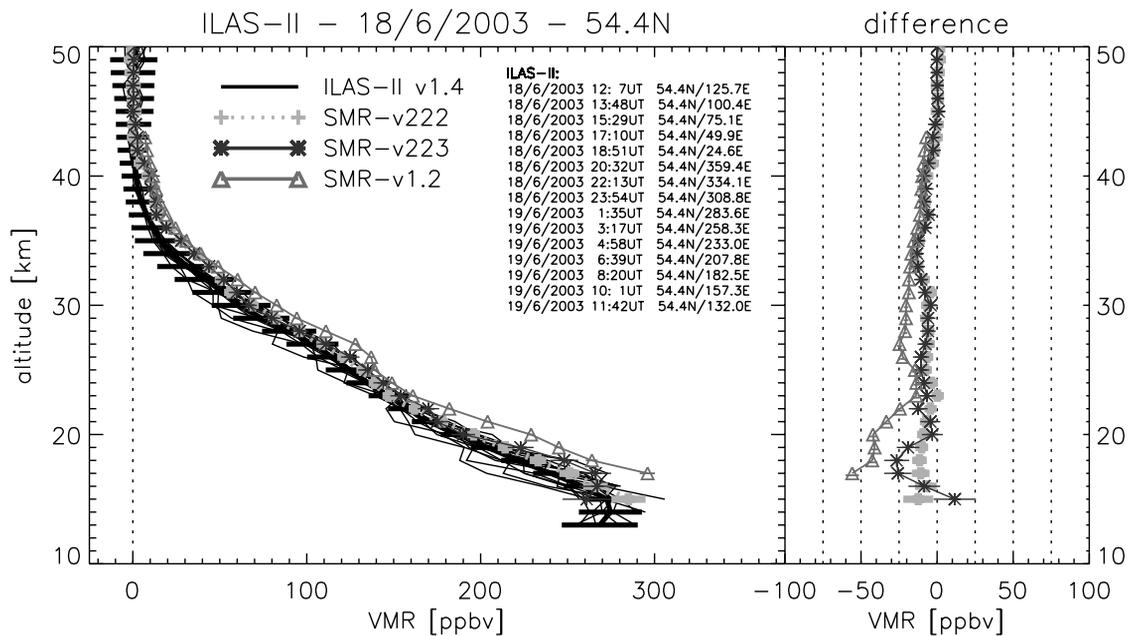
**Figure 9.** Comparison of Odin/SMR N<sub>2</sub>O with spaceborne ILAS-II infrared solar occultation measurements taken at northern middle latitudes on 18–19 June 2003 (1200–1200 UT). Odin/SMR measurements were averaged within a latitude band of  $54.4 \pm 2.5^\circ\text{N}$ . The plot shows the comparison of the zonal mean SMR profiles with the zonal mean ILAS-II profile (thick black line with  $1\sigma$  error bars). The thin black lines are the individual ILAS-II measurements.
