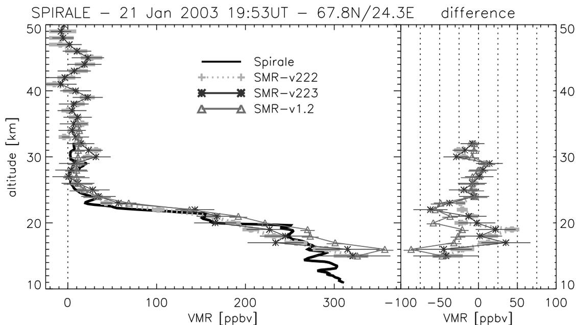
**Figure 3.** Comparison of Odin/SMR N<sub>2</sub>O with measurements of the balloonborne SPIRALE instrument taken at the edge of the Arctic polar vortex on 21 January 2003 over northern Scandinavia. The average SMR profiles used for the comparison with SPIRALE (averaged within  $\pm 1$  day,  $\pm 7.5^\circ$  in latitude,  $\pm 15^\circ$  in longitude), are based on three limb scans sounding air masses inside the polar vortex.
