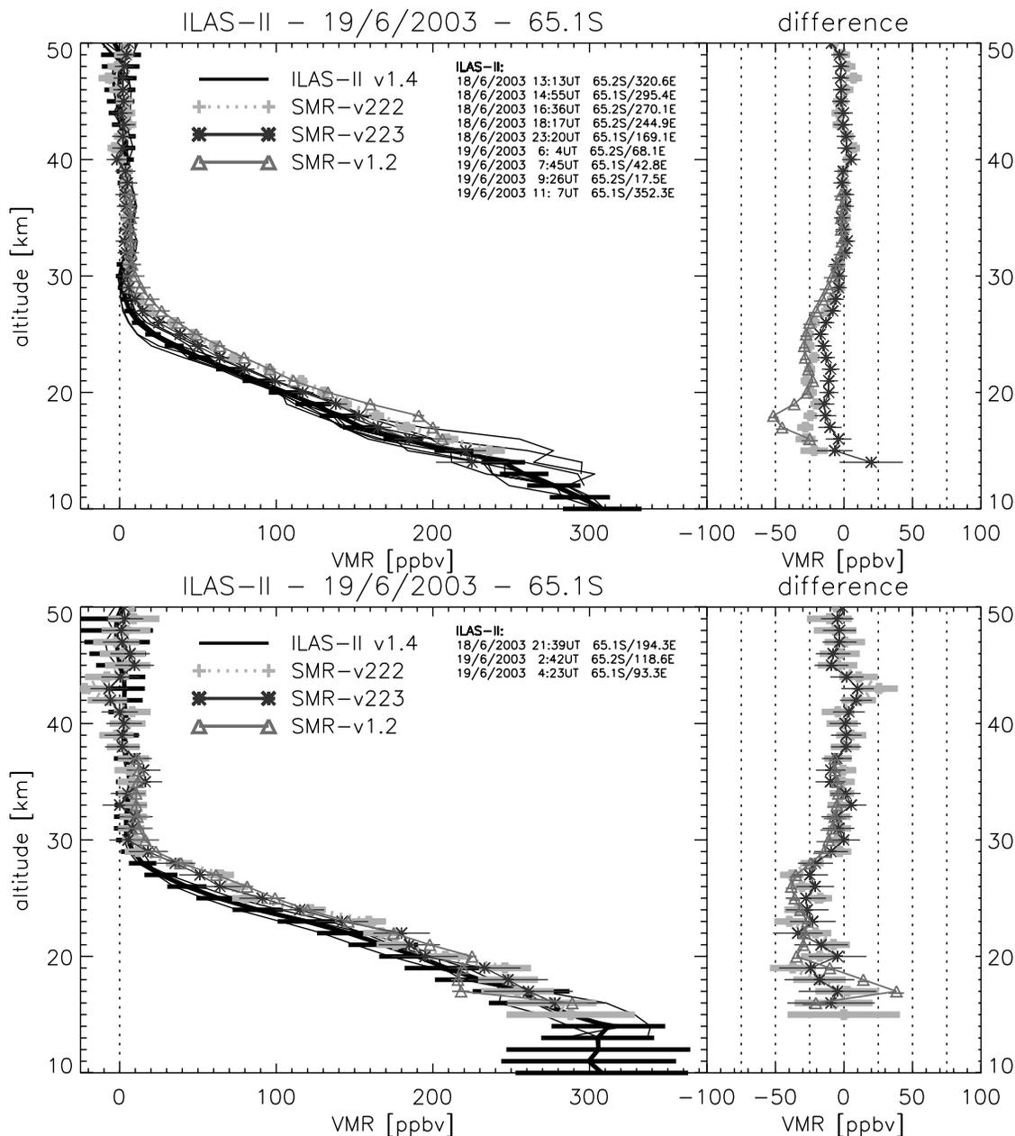
**Figure 10.** Same as Figure 9, but for Odin/SMR and ILAS-II N<sub>2</sub>O observations from 18–19 June 2003 (1200–1200 UT) at southern high latitudes in a latitude band around  $65.1 \pm 2.5^\circ\text{S}$ . (top) Comparison of measurements taken inside the Antarctic polar vortex. (bottom) Comparison of outside vortex averages.
