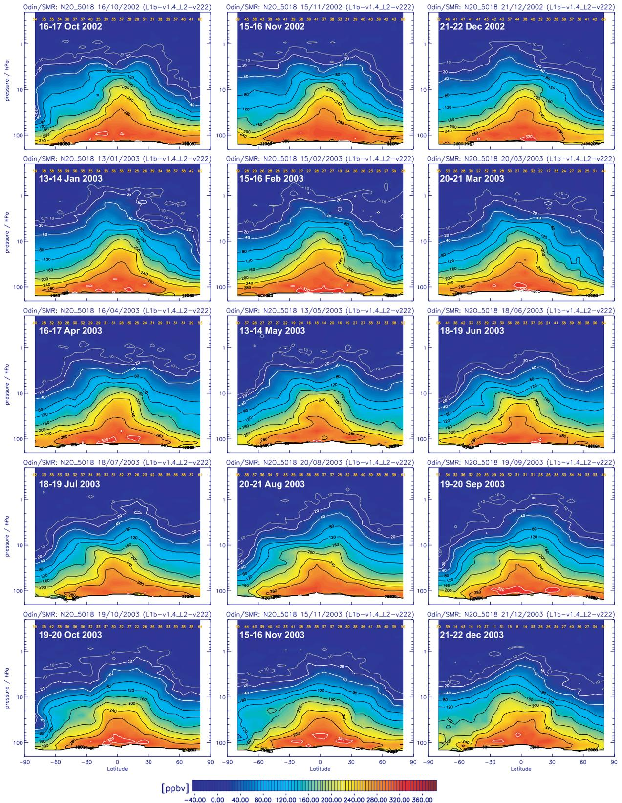
**Figure 15.** Global zonal mean N<sub>2</sub>O distribution derived from Odin/SMR measurements for selected observation days during a 15 month period from October 2002 up to December 2003 (version 222 data). Data are binned to 7.5° wide latitude intervals.
