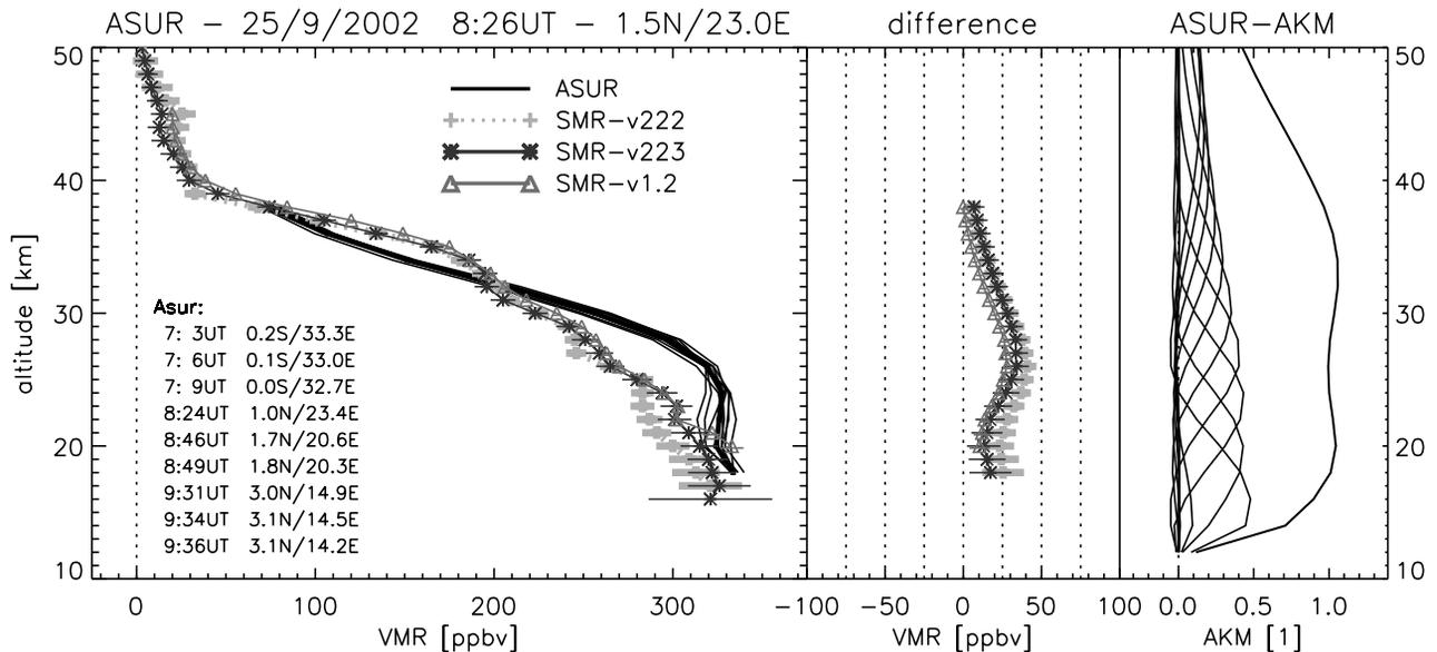
**Figure 7.** Same as Figure 6, but for measurements of the air-borne ASUR radiometer from a flight close to the equator performed on 25 September 2002. Ten individual SMR profiles within the usual coincidence limits were averaged for this comparison. To calculate the difference (middle), the unsmoothed Odin/SMR profiles (left) have been convoluted with the averaging kernel functions of the ASUR measurements (right).
