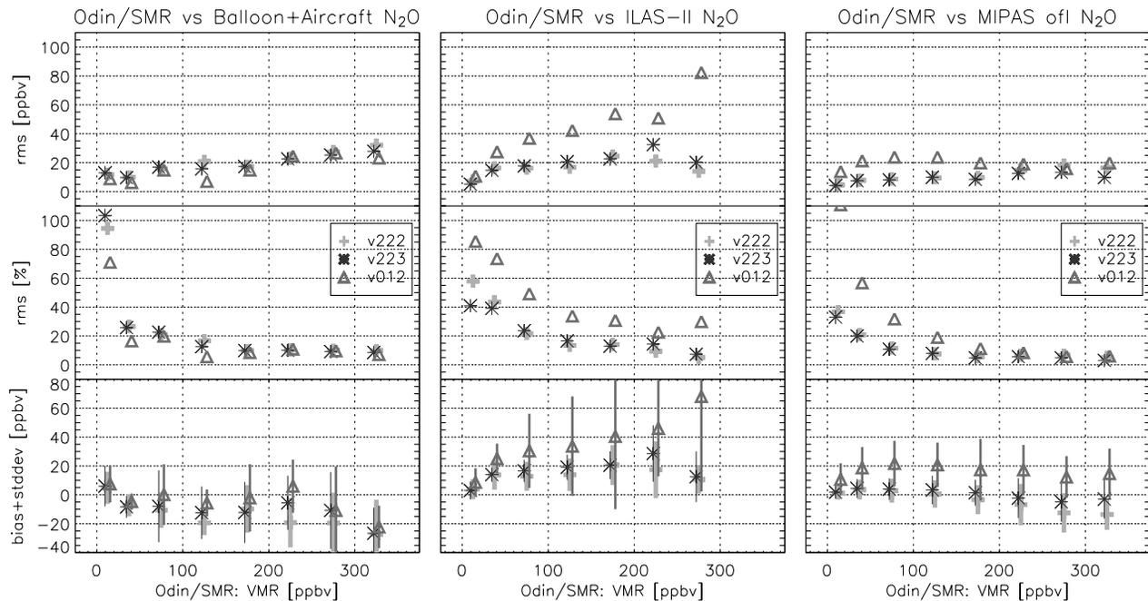
**Figure 16.** Differences between Odin/SMR N<sub>2</sub>O data (versions 222, 223, and 1.2) and correlative measurements. The top and middle panels of each part show absolute and relative root mean square deviations. The bottom panels show bias and corresponding standard deviation (bars). Data are binned to 50 ppbv wide intervals. (left) Airborne validation experiments. (middle) ILAS-II onboard ADEOS-II (level 2 version 1.4). (right) Envisat/MIPAS (off-line processor, version 4.61).
