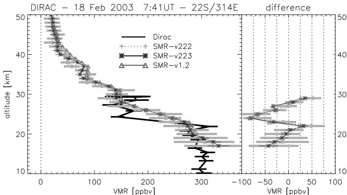
**Figure 5.** Comparison of Odin/SMR N<sub>2</sub>O with DIRAC measurements at low latitudes. The balloon was launched in Bauru (Brasil) on 18 February 2003. SMR data are averaged within  $\pm 1$  day,  $\pm 7.5^\circ$  in latitude and  $\pm 15^\circ$  in longitude with respect to the validation measurement (four profiles).
