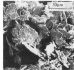
Fig. 8. Debris along the main crack flanks during a torsional test.
