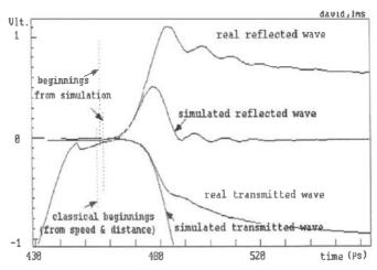
Fig. 4. Determination of the beginnings by elastic simulation.
