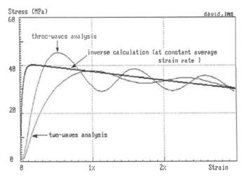
Fig. 9. Stress-strain curves from different analyses.
