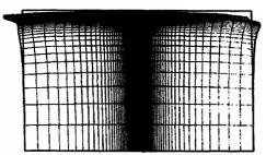
Fig. 2. Residual deformed mesh (  $\times$  100) after 1000 passes, for  $P_0/k_c$  = 4.76,  $\mu$  = 0. The total length is 26a.
