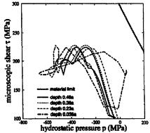
Fig. 6. Loading paths at different depths.
