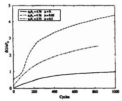
Fig. 3. Accumulated surface displacement for different values of  $P_0/k_e$  and  $\mu$ .
