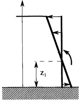
FIG. 6. Failure Mechanism without Circular Hinge
