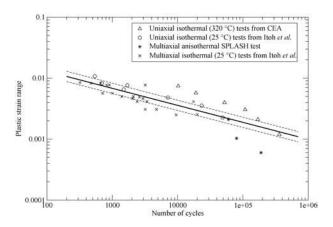
**Fig. 2** Manson parameter for the SPLASH test, the uniaxial isothermal tests from CEA<sup>3</sup> and the experiments from Itoh *et al.*<sup>11</sup>
