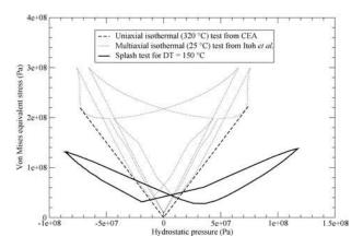
Fig. 5 Local hydrostatic pressure - Von Mises equivalent stress diagram for the SPLASH test, the uniaxial isothermal tests from  $CEA^2$  and the experiments from Itoh *et al.*<sup>10</sup>
