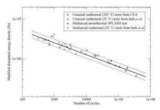
Fig. 6 Modified energy density parameter for the SPLASH test, the uniaxial isothermal tests from  ${\rm CEA^3}$  and the experiments from Itoh *et al.*<sup>11</sup>
