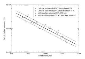
Fig. 4 Park & Nelson's fatigue parameter for the SPLASH test, the uniaxial isothermal tests from  $CEA^3$  and the experiments from Itoh et al.  $^{11}$
