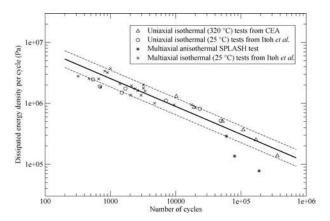
Fig. 3 Dissipated energy density parameter for the SPLASH test, the uniaxial isothermal tests from  $CEA^3$  and the experiments from Itoh *et al.*<sup>11</sup>
