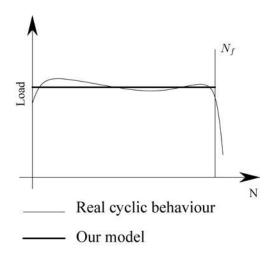
Fig. 1 Cyclic behaviour of 304L stainless steel.
